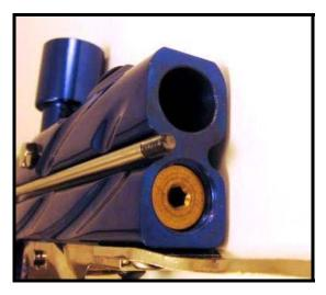
Your marker will look like this once the Bolt, Bolt Pin, Cocking Rod, and Back Block have been removed.
